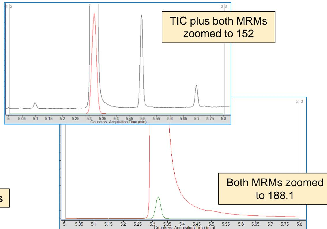
The spectrum is p-chlorobiphenyl. The MRM shows that the collision cell is working because 188.1 is essentially gone.
