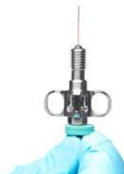
Injection Port Self-Tightening Column Nut
