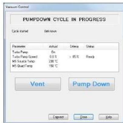
11. When prompted, turn on the GC/MSD interface heater and GC oven. Click on OK when you have done so. The software will turn on the ion source and quadrupole heaters. The temperature setpoints are stored in the current tune file (\*.u).
