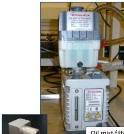
Oil mist filter mounted on Edwards RV5 pump
