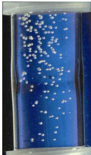
The apparatus' 300 mL vessels typically contain a working volume of 200 to 275 mL vessel volume, avoiding overflowing of the media during periods of higher reciprocation rate. The operational minimum is about 150 mL vessel volume. A wide range of products may be tested in the apparatus
