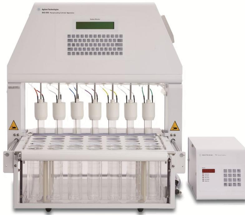
Performing the test: When the test begins, the reciprocating cylinders descend slowly into the first row of the vessels. Then the reciprocating motion starts. After the programmed time for this row expires, the reciprocating cylinders rise above the vessels to drain for a programmed time, and automatically move to the next row. Then the reciprocating process is repeated in the vessel containing the next media.
