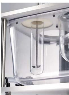
The 708-DS makes conversion to a smaller volume simple. A conversion kit for each location includes an adapter ring and evaporation cover. If the system is automated, the manifold is easily adjusted to accommodate the smaller vessel size. Mini TruAlign vessels (100, 200, or 250 mL) and mini-basket or paddle shafts complete the conversion. The 100 mL vessel allows for dissolution in as little as 50 mL.
