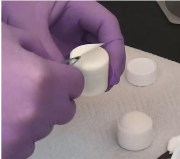
Attaching the surface area ring: The surface area ring controls the surface of the membrane to standardize the release area. These rings are available in three sizes; 4, 2 and 0.5 cm<sup>2</sup> with the 4 cm<sup>2</sup> size being the most common (shown following):
