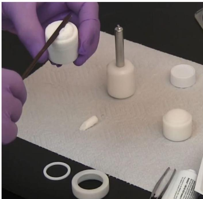
Applying the membrane: The membrane must be presoaked in the receptor medium for at least 20 minutes. The membrane is then removed from the medium with tweezers taking care to only handle the edge and not damage the surface of the membrane. The membrane is then rolled onto the surface of the product to avoid the entrapment of air.
