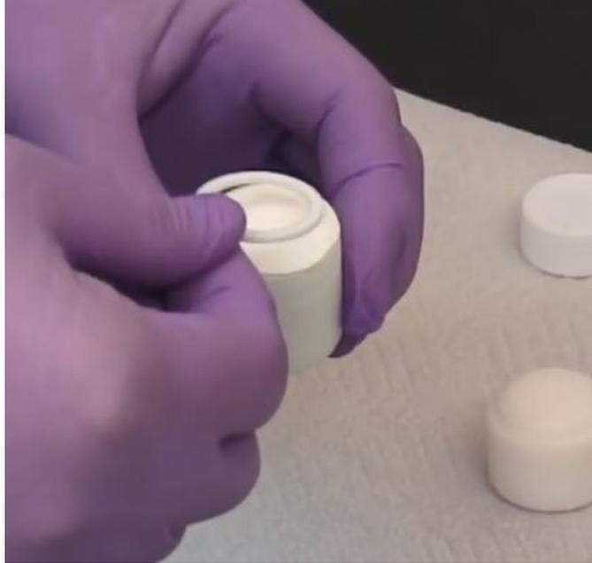
Attaching the retaining ring: The surface area ring is held in place by a retaining ring that is screwed onto the cell body until a small amount of resistance is felt:
