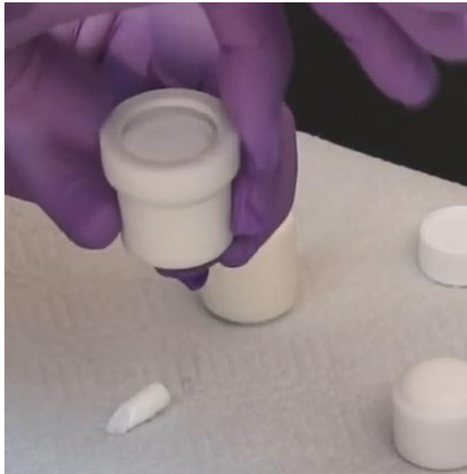
Adjusting the centering ring: The centering ring is adjusted with an alignment tool that may also be used to set the height. The alignment tool is wiggled into place and the groove in the tool places the centering ring exactly in the middle of the cell. Once the centering ring is centered, the retaining ring is tightened slightly. Over-tightening may result in damage to the membrane. The alignment tool should remain in place during the adjustment step:
