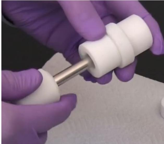
**Ready for testing:** After tightening, remove the tool and the Enhancer Cell is prepared and ready to test. Prepare the additional 5 cells for the **drug release** testing:
