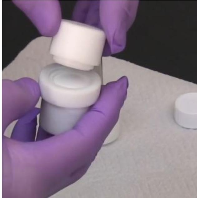
Adjusting product contact to the membrane: The product must be pushed up against the membrane while the alignment tool is in place. This is accomplished with an adjustment tool that looks similar to a screwdriver. Once the tool is inserted, about one-quarter turn clockwise is applied to press the product against the membrane.
