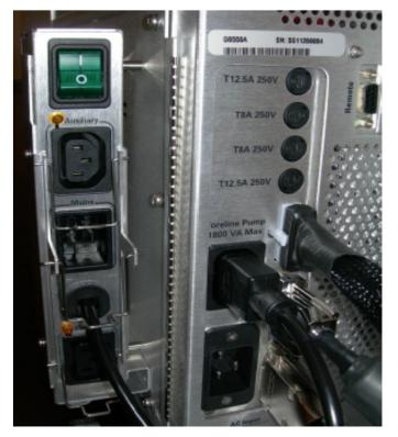
2. Turn off Pump Expander box\* Installed on: 6420, 6460C, 6470, 6490, 6495
