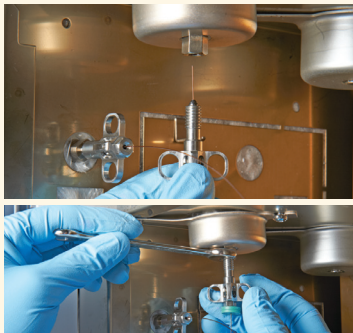
Inlet/Detector – narrow end of the ferrule faces away from the nut.
